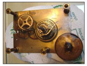
The clock was found to have two faults; the original main spring was broken at the winding arbor end and found to be very tired. The escape wheel pinion was also badly worn, the associated wheel had been moved to rectify this once before during a past repair, and so this could not be done again. The escape wheel pivots were very badly worn and so the decision was made to fit a new pinion and arbor. The old parts were returned to the owner to be kept with the clock as part of its history.
