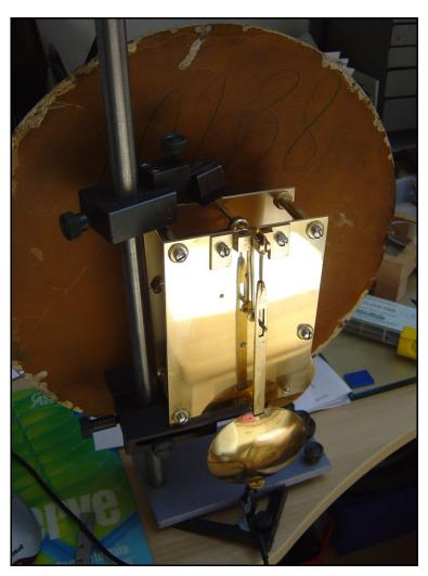
The clock is now assembled, the lubrication has been done and the rate is being adjusted with a Microset computer clock timer
