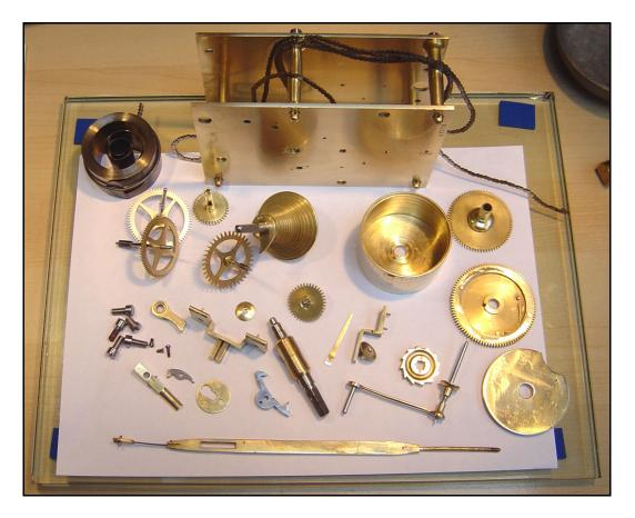
The clock has now been repaired and ultrasonically cleaned and is ready for assembly.
