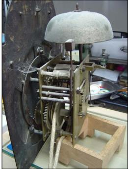
The dial shows the typical damage caused by repeated polishing with metal polish. This over a period of time reduces definition of engraving and as the metal polish builds up it causes corrosion and verdi gris. The hand is original and fortunately we had the pieces to make a good repair.
