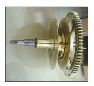
Corrosion and metal polish now removed, the chapter ring re-silvered. The movement had the usual pivot wear and required some bushing.
