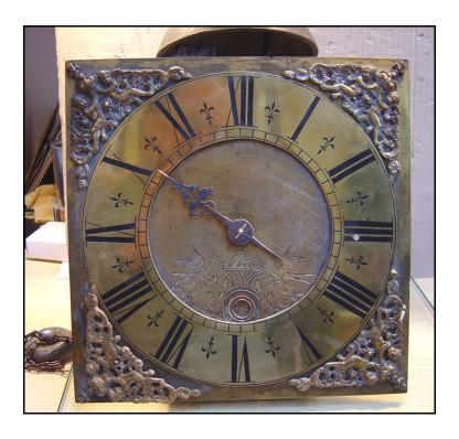
This clock is a provincial brass dial clock (10 inch sq face) with a posted frame movement and made about 1725. The clock has no makers mark but is well made.
