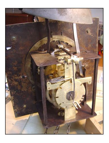
The movement after the restoration work was completed. The pinions in this clock do show signs of wear but this is to be expected and is not yet at the stage that action needs to be taken. Several pivots were worn, these were repolished, yellow cast brass bushes were then made and fitted as required
