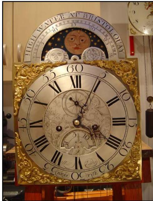
The dial has been re silvered and lacquered, the black wax being replaced as required. The tidal dial plaque had been damaged and poorly repaired in the past. One of the new replacement hands being sculpted from steel
